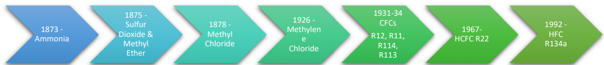
Timeline of the common use" of refrigerants in a Vapour Compression Cycle.
